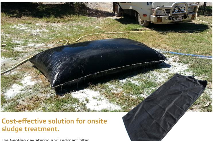
The GeoBag dewatering and sediment filter bags are perfect for pumping and filtering sediment laden water. Our standard rage of dewatering bags provide a simple yet effective method of removing heavy particles (>180 microns) from excavation water allowing silt free water to be released from the bag.
