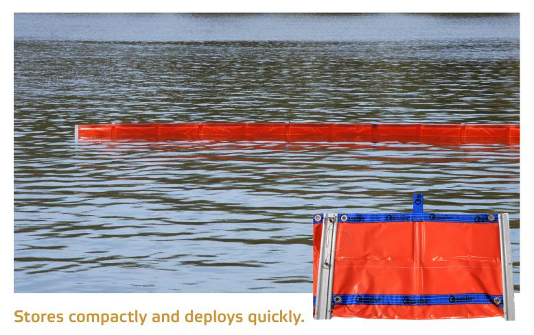
Fence Booms are a fence like barrier designed to deflect or contain oil and floating debris. The fence boom is constructed using square and flat sections allowing it to be stored in bags, cages or reels. This PVC fence style oil containment boom stands up higher in the water. This particular boom is better suited to calm or sheltered waters.
