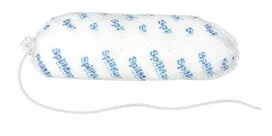
Manufactured with UV resistant tough spun bonded outer mesh encasing a polypropylene particulate. Each boom features a nylon rope that allows it to be secured and then easily retrieved. A bilge boom can absorb up to 2L per saturation. Even when fully saturated, these durable booms will remain intact and float on water.
